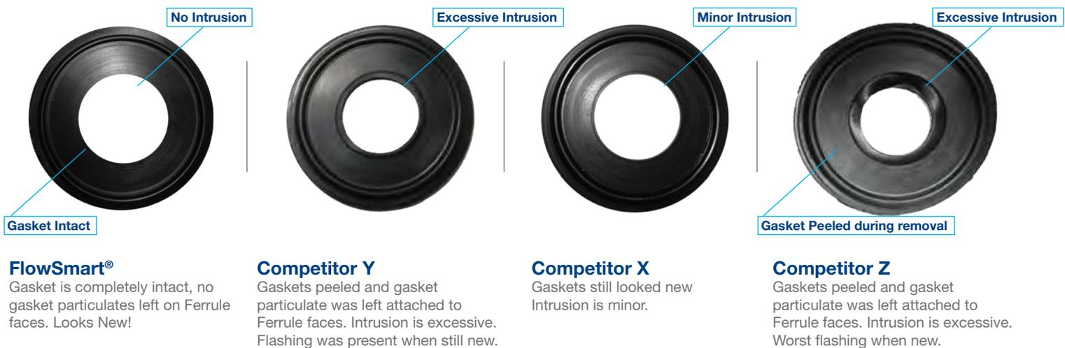
The gasket study was done for FlowSmart. It was a blind study that revealed very definitive and consistent details. The criteria of the tests were as follows:
